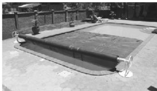
Covers are effective solution to raising pool temperatures as they work by simple principle of eliminating evaporation and thus heat loss. Covers are made from specifically formulated Ultra Violet (UV)protected PVC material and the moulded air bubbles provide effective heat insulation. Covers are manufactured to the specific pool size and are available with rollers for ease of covering and removal
